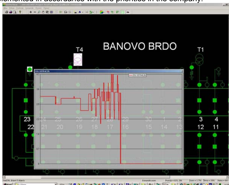
Figure 4 - Load diagram displayed over the substation scheme
